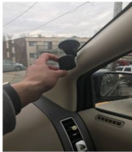
Step 2: Affixed magnetic holder onto the windscreen to hold the tablet
